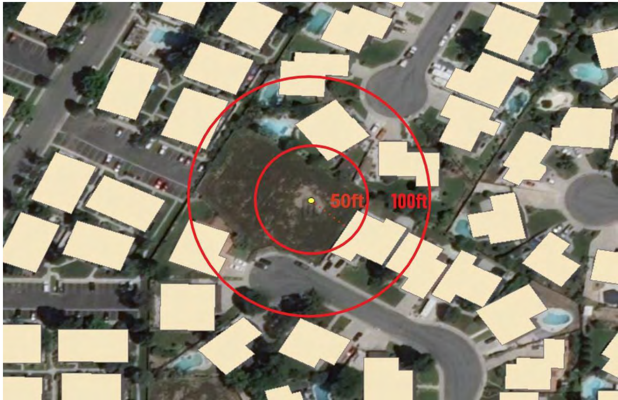
Figure 7.10. Active-producing well (yellow marker) near Bakersfield depicting the hyperlocal proximity to nearby homes (tan color). Radial distances from the well are depicted in red approximately 50 ft and 100 ft from the wellhead. Distances between buildings and their nearest well as shown here were used to create the frequency histogram as shown in Figure 7.11 .
