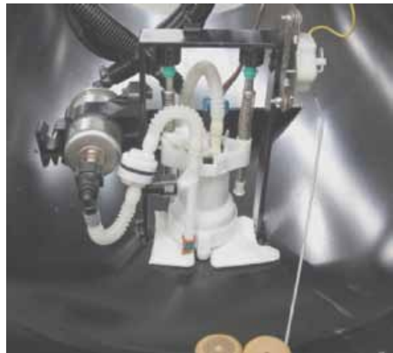
Figure 96. Roush LPI tank internal components
