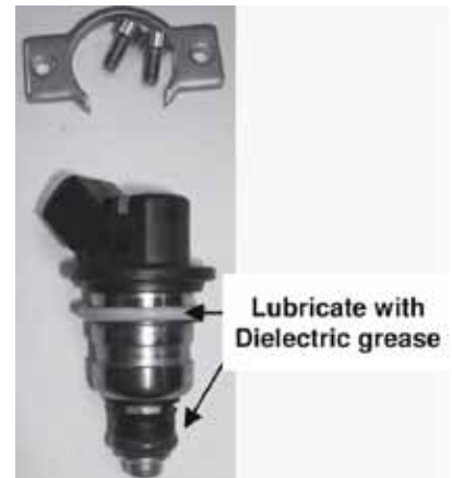
Figure 87. Replacement injector installation
