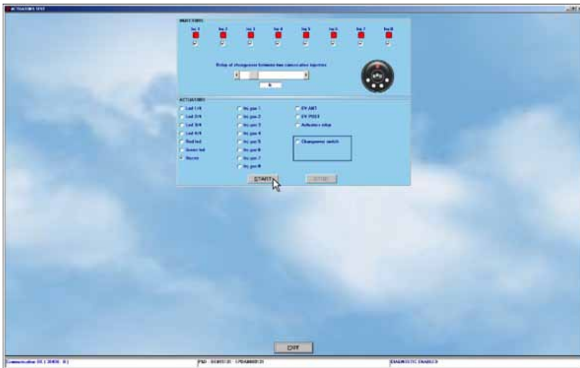
Figure 29. Actuator screen with injector and solenoid test buttons
