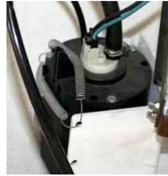
Figure 60. Internal tank view of fuel-pump housing
