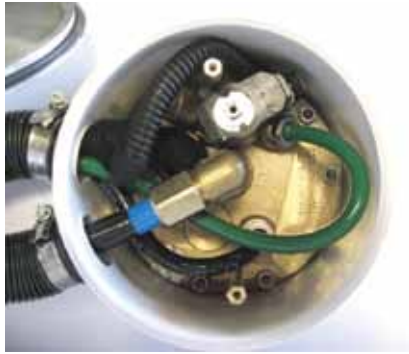
Figure 59. Outside view of tank multivalve
