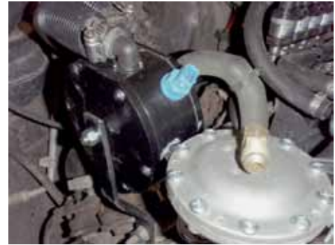
Figure 114. Prins vaporizer with primary fuel filter
