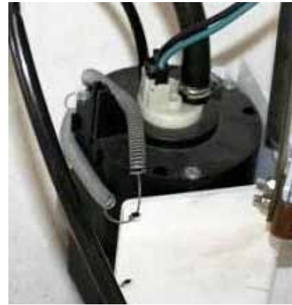
Figure 78. Fuel-pump electrical connection
