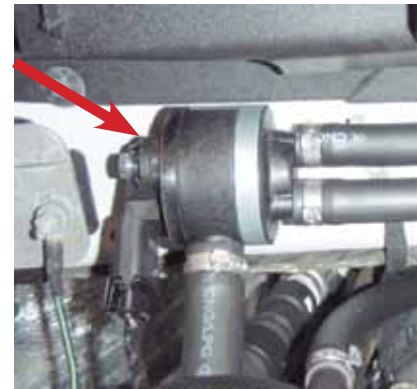
Figure 115. Pressure and temperature transducer combined with the secondary fuel filter
