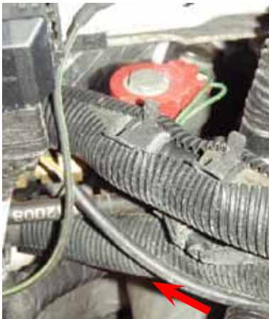
Figure 14. Primary (liquid) filter. The primary or liquid filter is directly below the fuel solenoid, just behind the hose indicated by the red arrow. It may be serviced on the vehicle.
