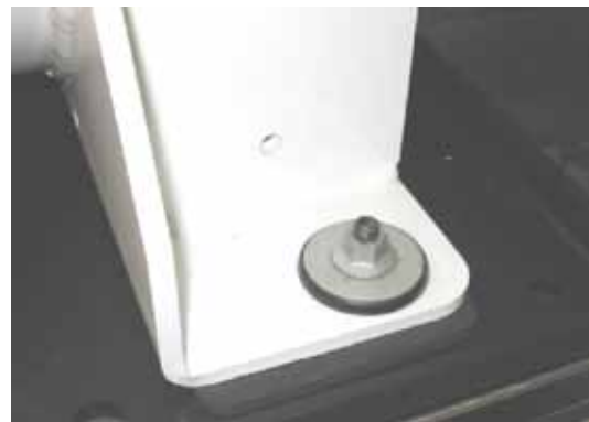
Figure 93. Tank hold-down nuts
