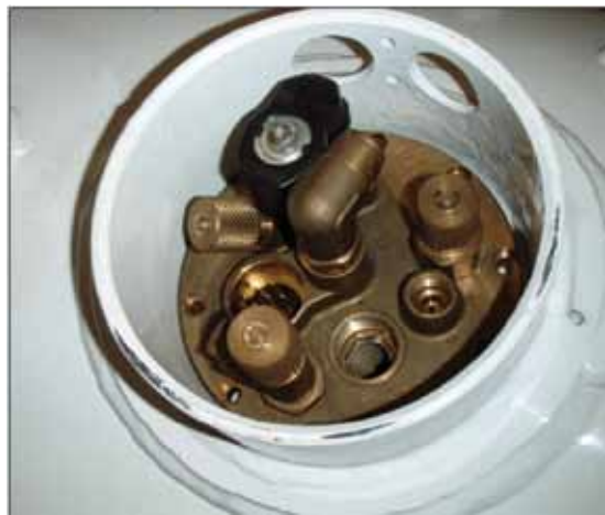
Figure 63. Early-style multivalve with integrated pressure-relief valve
