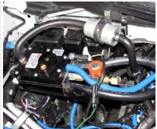
Figure 41. 2010 F-150 vaporizer location
