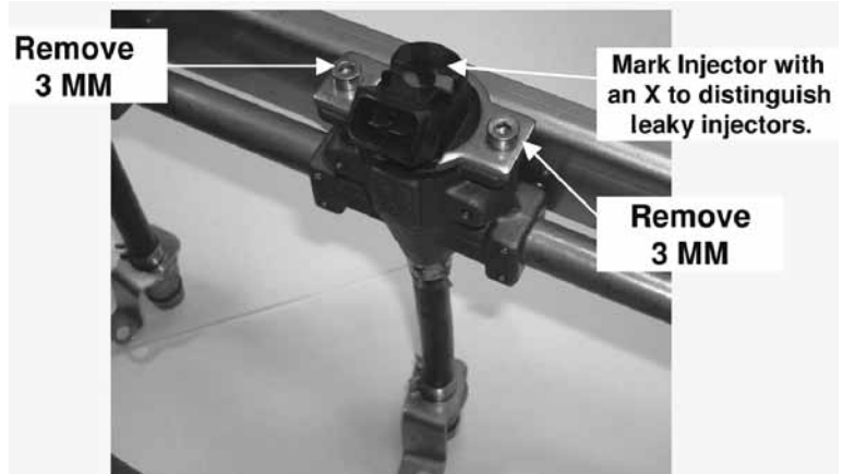
Figure 56. Injector retaining bracket screws
