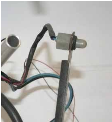
Figure 61. Internal tank view of fuel-level photocell
