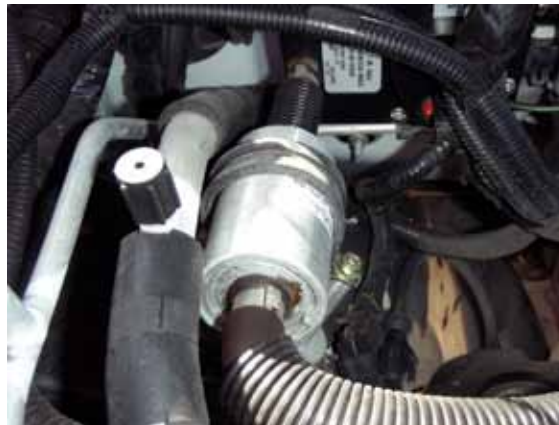
Figure 15. Secondary (vapor) filter. The secondary or vapor filter is located in the low-pressure hose between the vaporizer and the tee that feeds the two injector rails. It may be serviced on the vehicle.
