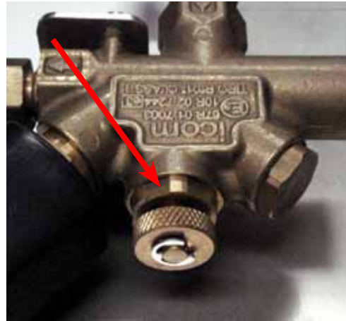
Figure 54. Fuel pressure regulator shutoff knob
