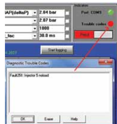
Figure 110. Display showing trouble code, fuel and fault description
