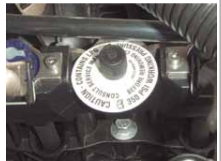
Figure 86. Tank pressure test port
