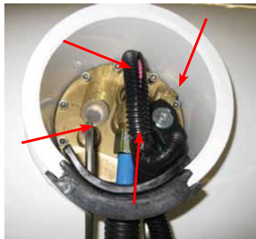
Figure 91. Multivalve fuel lines, wiring and shutoff knob
