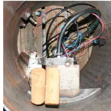
Figure 62. Internal tank view showing the fuel-level gauge floats, photocell, and fuel-pump housing
