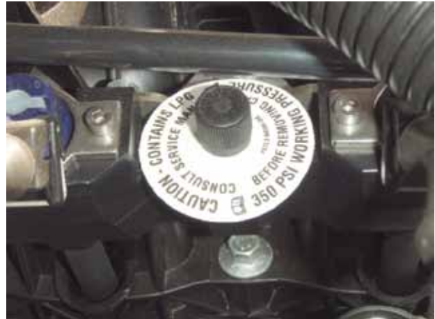
Figure 84. Tank pressure test port
