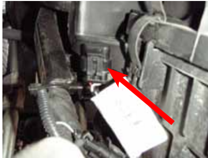
Figure 18. Diagnostic connector secured to coolant overflow bottle
