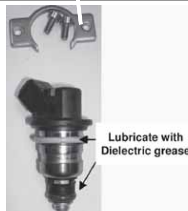
Figure 58. Replacement injector installation
