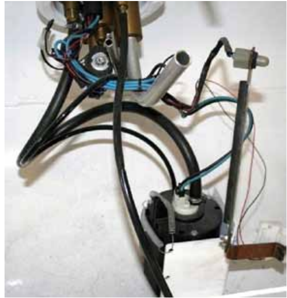
Figure 77. Fuel-pump housing removal
