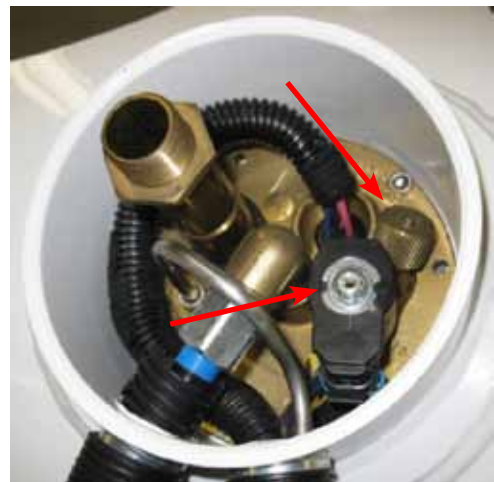
Figure 88. Manual service valve E-clip removal
